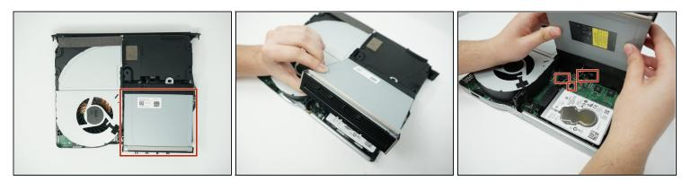
• Flip the disk drive up. The three plugs underneath (outlined in red in the third image) don't need to be unplugged.
