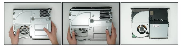
• Grab the sides of the Xbox One X bottom metal case in the middle by two hands and lift up vertically to remove the bottom metal case.
