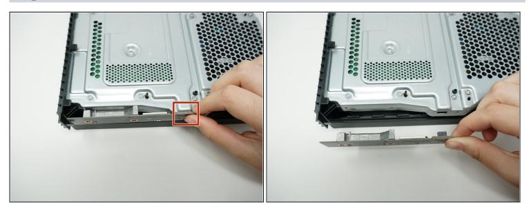
• Hold the circuit board tightly by two fingers and pull it straight off towards you. Make sure to keep it level.
