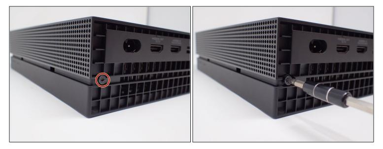
• Use a T9 screwdriver to unscrew (counter-clockwise direction) the black 13mm long screw circled in red from the back side to the lower left of the power connector.
