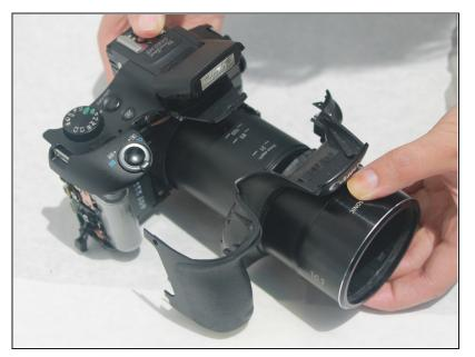
Remove the front cover by pulling along the lens housing while holding the body of the camera.
