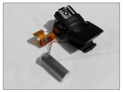
Once the above steps are completed, gently pull the flash assembly from the device and snap out the capacitor located on the front side of the camera
