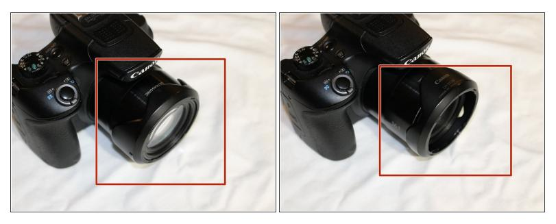
Remove the sunshade located on the front of the lens by twisting it 90 degrees in either direction, then pull straight off the lens.
