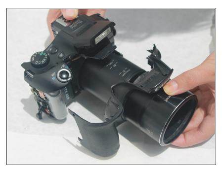
Remove the front cover by pulling along the lens housing while holding the body of the camera.
