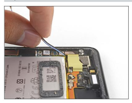
Carefully de-route both antenna cables and move them away from the charging assembly.
