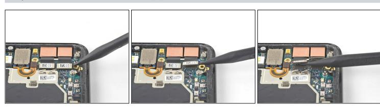
Use the point of a spudger to pry up and disconnect the connector for the camera(s) you are replacing.
