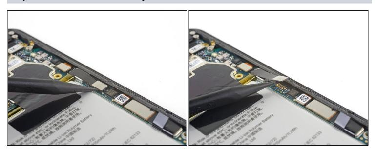
Use the point of a spudger to pry up and disconnect the battery press connector from its socket near the right edge of the phone.
