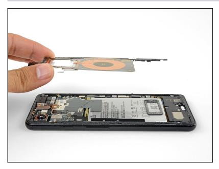
• Lift up and remove the wireless charging coil.
