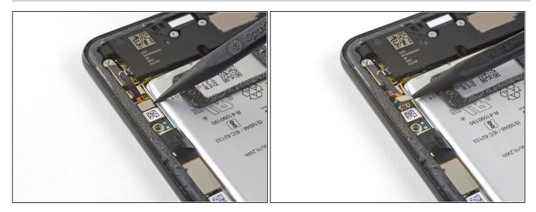
Use the point of a spudger to pry up and disconnect the loudspeaker connector from its motherboard socket near the right edge of the phone.
