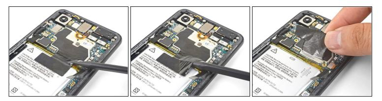
⚠ Whenever you use the spudger near the battery, be very careful not to puncture the battery.
