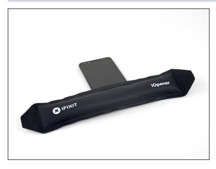
Heat an iOpener and apply it to the bottom of the phone for one minute.
