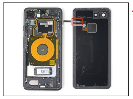
⚠ When inserting an opening pick above the power button, be careful not to insert the pick too deeply, or you will damage the fingerprint sensor cable.
