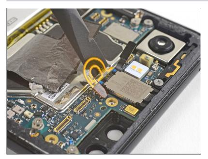
Use the flat of a spudger to carefully pry up and bend the earpiece speaker's flex cable upwards, out of the way of the motherboard.
