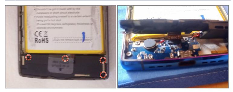
• Remove the screws at the bottom of the phone and carefully lift up the black speaker unit. Underneath is a small circuit board. Be careful not to break the metal braid joining the speaker to the phone.
