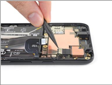
• Use the pointy end of a spudger to pry up and disconnect the camera cable from the motherboard.
