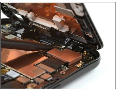
Use a spudger to pry up and detach the proximity sensor cable from the motherboard.
