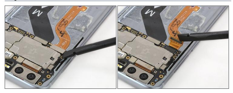
• Use a spudger to pry up and disconnect the display flex cable.
