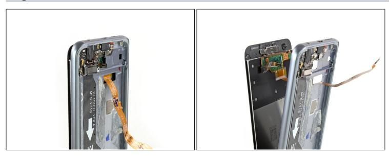
• Make sure the display flex cable does not stick to the frame and carefully thread it through the gap at the bottom of the frame.
