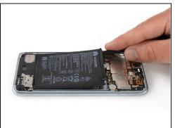
Insert the flat end of a spudger at the top left corner of the battery and pry the battery up.
