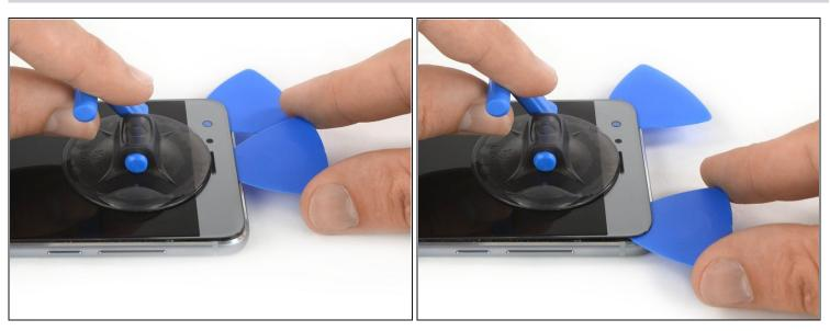
Insert a second opening pick and slide it to the top right corner of the phone.
