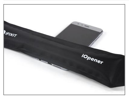
Apply an iOpener to the bottom end of the display to soften the adhesive beneath the loudspeaker.
