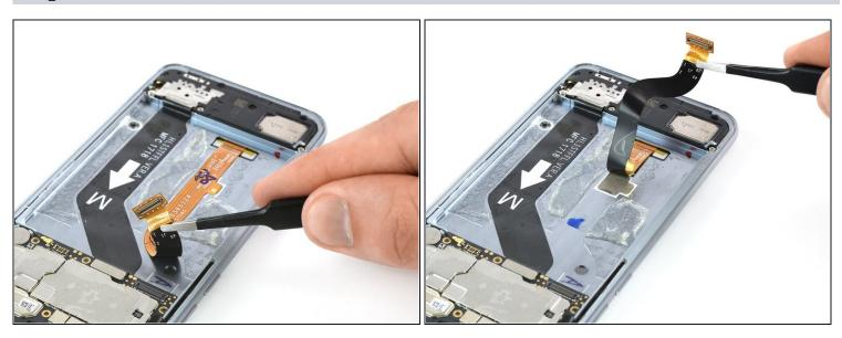
• Use a pair of <u>tweezers</u> to peel the display flex cable off the frame.
