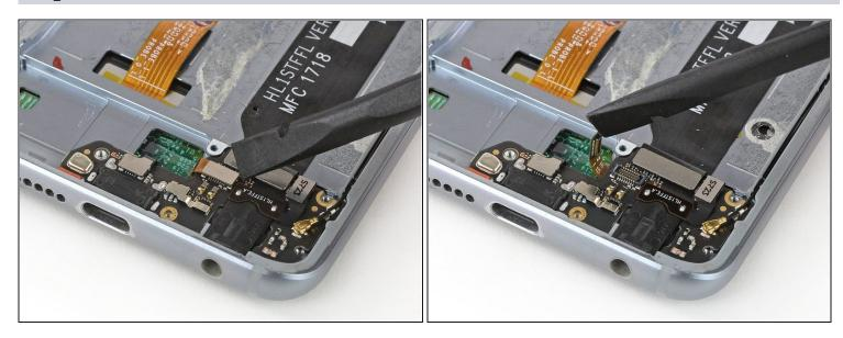
• Use a spudger to pry up and disconnect the home button flex cable located at the bottom right of the phone.
