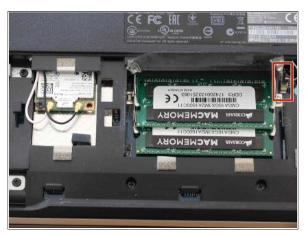
Use the flat end of a spudger to disconnect the connector marked in the photo.
