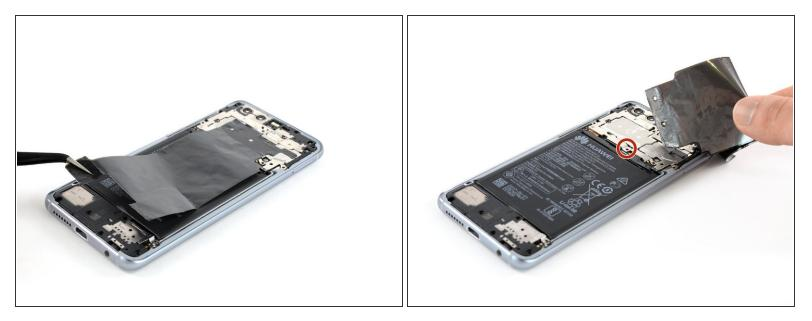
• Carefully peel up the black thermal foil and remove it completely.
