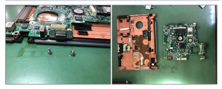
• Remove the screws to remove the motherboard.
