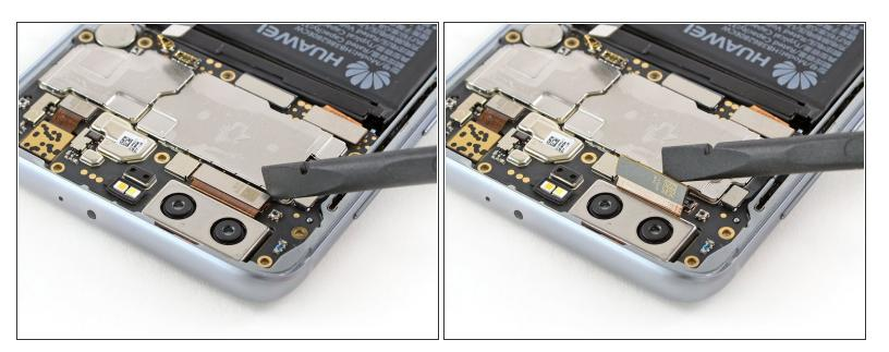
Use a spudger to pry up and disconnect the rear facing camera flex cable.
