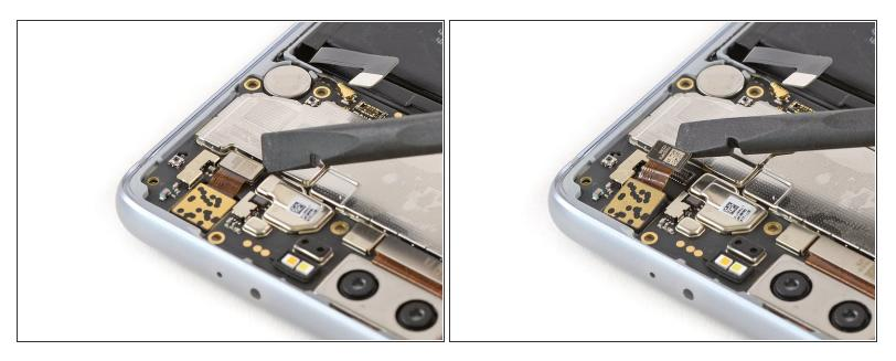
• Use a spudger to pry up and disconnect the front-facing camera flex cable.
