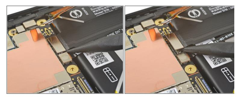
Use the point of a spudger to pry up and disconnect the interconnect flex cable from its motherboard socket.
