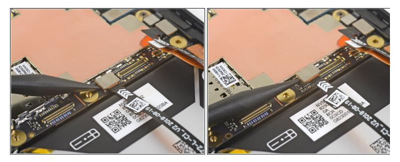
• Use the point of a spudger to pry up and disconnect the left squeeze sensor cable connector from its motherboard socket.
