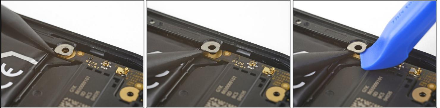
ⓘ The next two steps show how to loosen the right squeeze sensor bracket enough to free the loudspeaker pinned underneath it.
