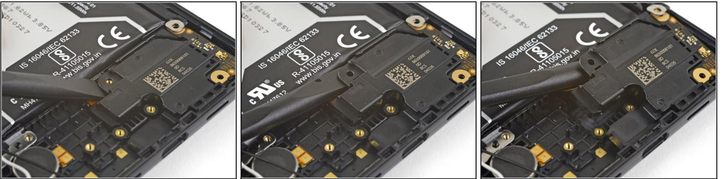
ⓘ The loudspeaker itself is adhered to the phone frame near the right edge of the phone.
