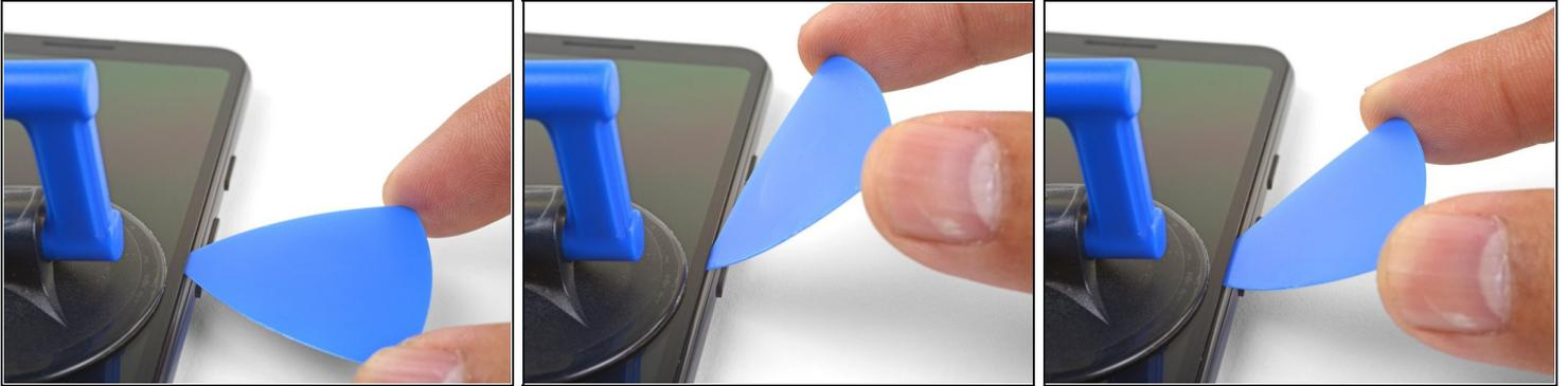
ⓘ This step shows how to insert the pick without damaging the OLED panel. Do this before you slice either long edges of the phone.
