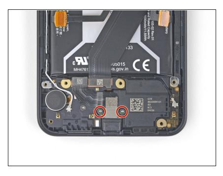
Remove the two 3.3 mm T3 screws securing the USB-C port.
