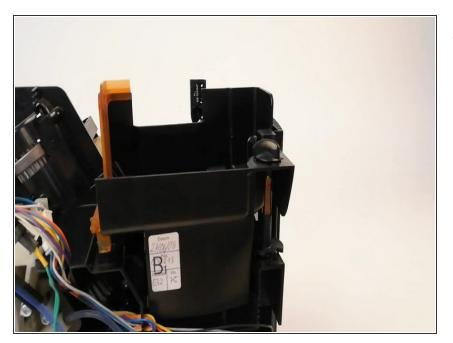
Remove the grinding degree adjustment axle by using pliers to pull it upwards.
