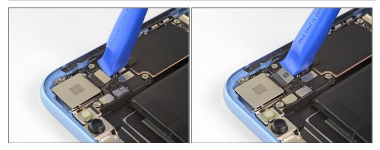
• Use an opening tool or fingernail to disconnect the camera cable connector by prying it straight up from its socket.
