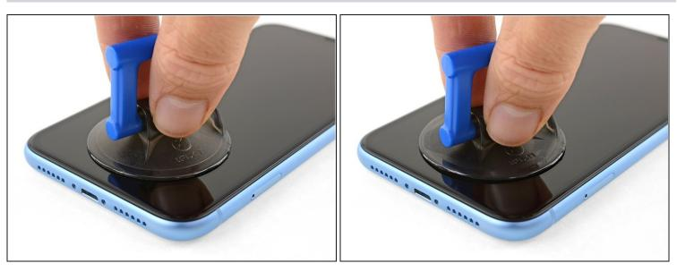
• If you're using a single suction handle, apply it to the bottom edge of the phone, while avoiding the curved portion of the glass.
