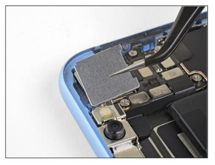
• Lift the camera cover straight up and off of the camera.
