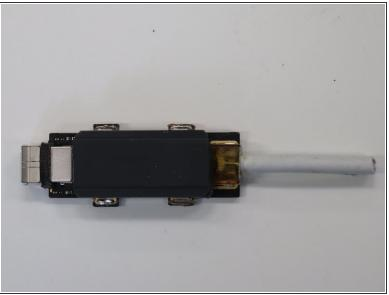
Both sides of the PCB are covered by thermal adhesive.
