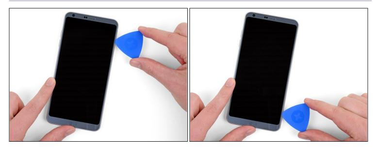
• Slide your opening pick down the final long edge of the phone to separate the last of the adhesive holding the screen in place.
