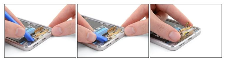
• Use the flat end of an opening tool to pry up the USB-C / mic assembly and remove it from the phone.
