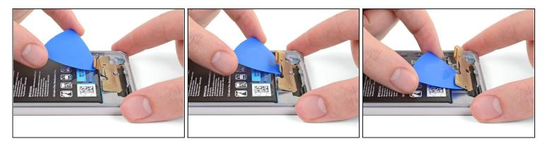
Slide an opening pick under the display cable to separate the adhesive holding it in place.
