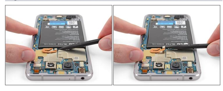
• Use a spudger to pry up the press connector at the end of the battery's ribbon cable, disconnecting the battery.
