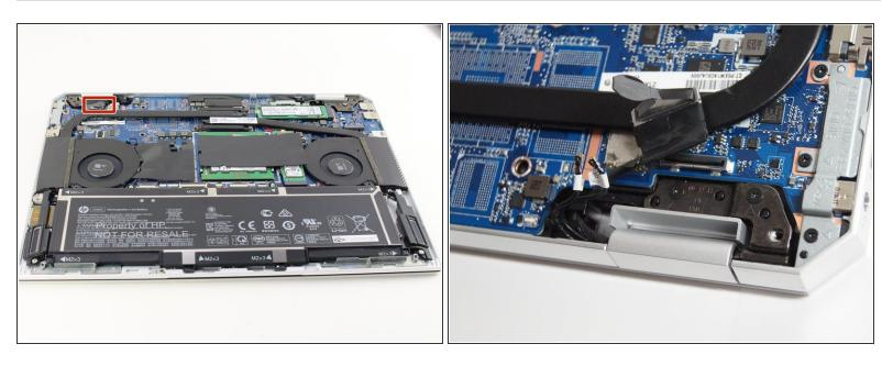
Remove the camera cable from the board as indicated.
