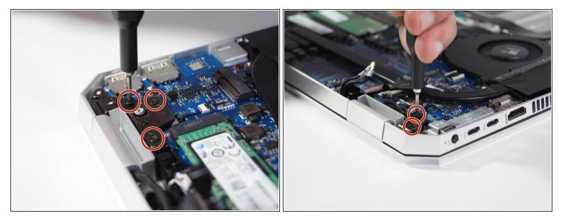
Remove the five black 5 mm screws from the screen brackets near the screen hinges using the Phillips #00 screwdriver.
