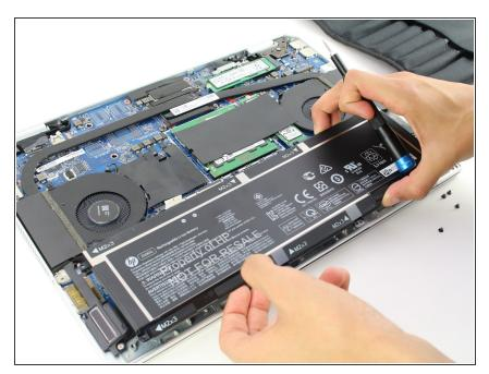
Grip the battery by the edges and lift it out of its housing.
