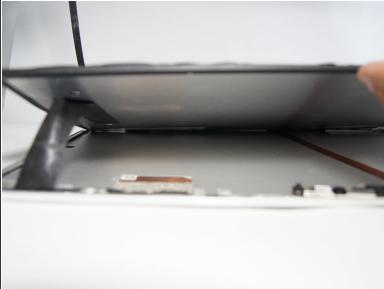
Peel away and remove the screen from the silver laptop shell.
