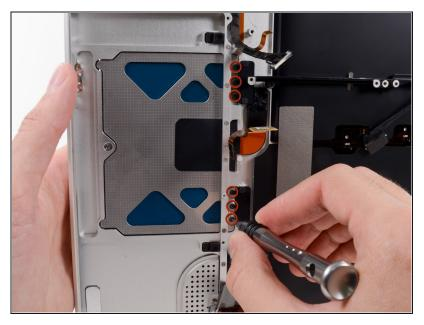
While holding the edge of the trackpad closest to the logic board with one hand, remove the six 1.3 mm Phillips screws securing the two brackets to the trackpad.
