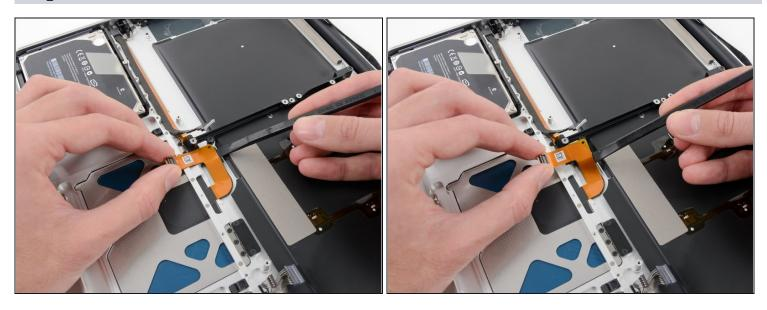
• Insert the flat end of a spudger underneath the trackpad ribbon cable and gently peel it up from the adhesive securing it to the upper case.
