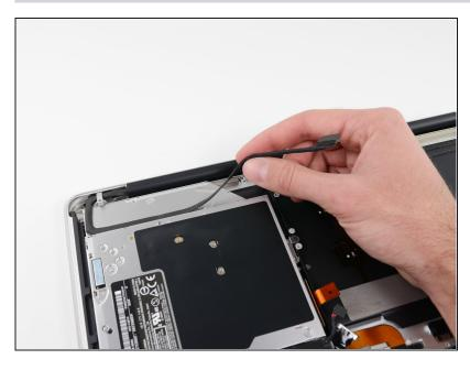
Deroute the camera data cable from its channel on the optical drive.
