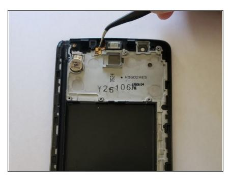
Still using the tweezers, remove the front speaker unit by lifting up on the ribbon cable connector.
