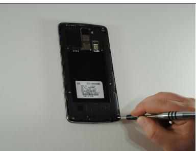
Using the JIS #000 screwdriver, remove the eleven 4mm screws around the mid-frame.
