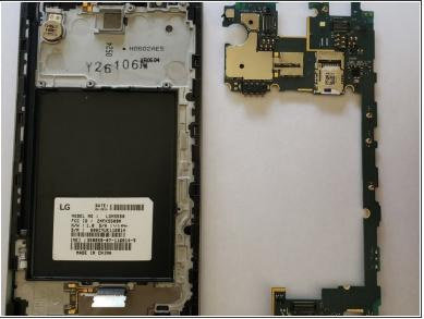
With the mainboard now free, carefully remove it and set it to the side.
