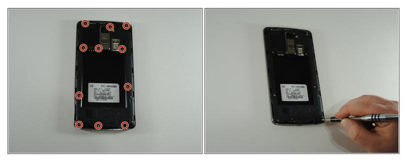
▶ Using the JIS #000 screwdriver, remove the eleven 4mm screws around the mid-frame.
