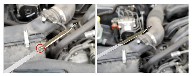
Remove the dipstick and clean it. Then reinsert it and remove it again and ensure the second dot on the end of the dipstick is touched by oil.
