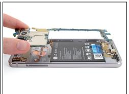
• Grab the motherboard by the top end (the end with the cameras) and gently lift it up and out of the phone.
