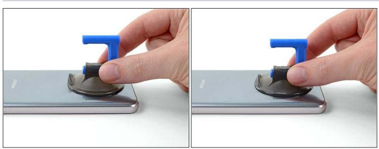
• Secure a suction cup to the rear panel, as close to the heated edge as possible.
