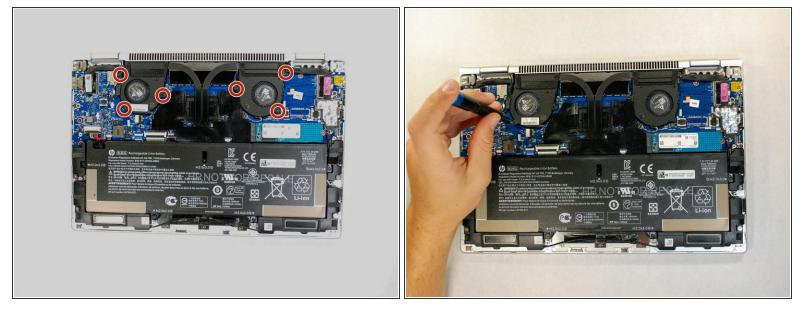
• Use the Phillips 0 screwdriver to remove the six 3mm Phillips screws from the fan assembly.
