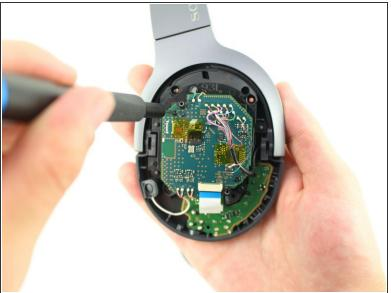
• Use the JIS #00 Screwdriver to remove the 2 6.4mm screws holding in the motherboard.
