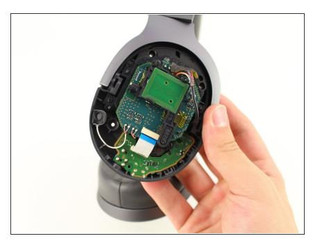
Gently remove the old motherboard from the bracket assembly and replace and resolder motherboard.
