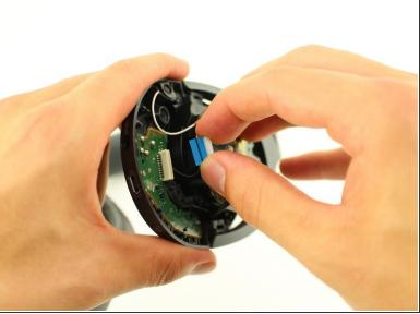
Disconnect the white ribbon cable by gently tugging on the white connector while holding the motherboard carefully in place.
