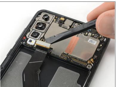
Use the flat end of a spudger to pry up and disconnect the display flex cable at the bottom left of the motherboard.
