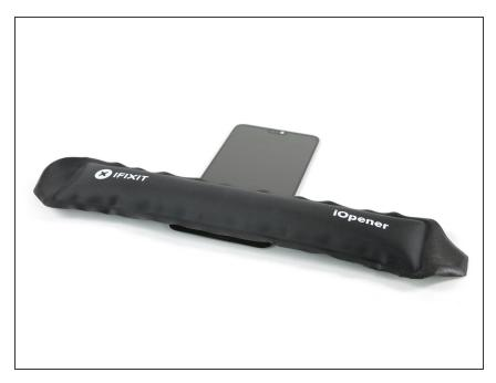
Use an iOpener to loosen the adhesive beneath the home button.
