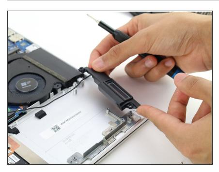
Lift the speaker up to fully remove it.
