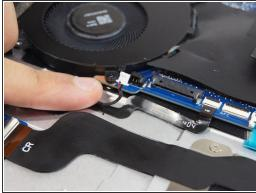
• Use the iFixit opening tool to remove the speaker cable for the other speaker. Make sure to apply moderate pressure on the sides of the cable to loosen it.
