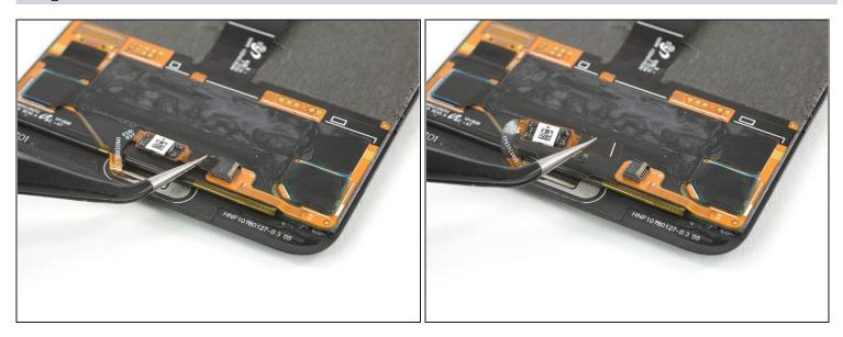
• Use a pair of tweezers to gently pull the home button flex cable out of its ZIF connector.
