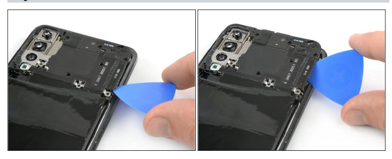
• Repeat the previous process on the right side and twist the opening pick to pry up the motherboard cover.
