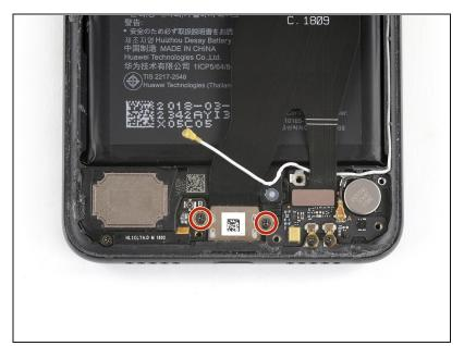
Remove the two Phillips #00 screws (3.4 mm length) on both sides of the USB C port.
