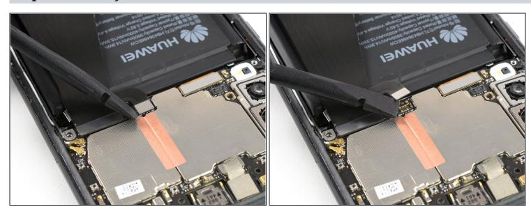
• Use the flat end of a spudger to pry up and disconnect the battery flex cable.
