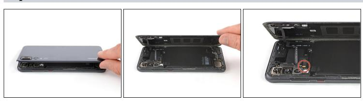
• Carefully lift the rear glass until you can reach the connector of the proximity sensor flex cable next to the rear camera assembly.
