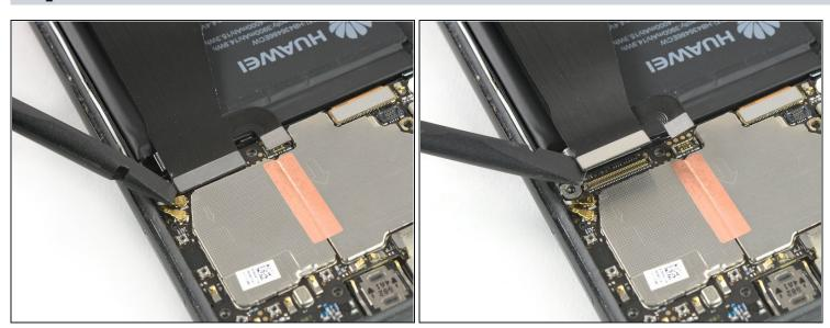
Use the flat end of a spudger to pry up and disconnect the upper end of the interconnect and charging port flex cable from the motherboard.
