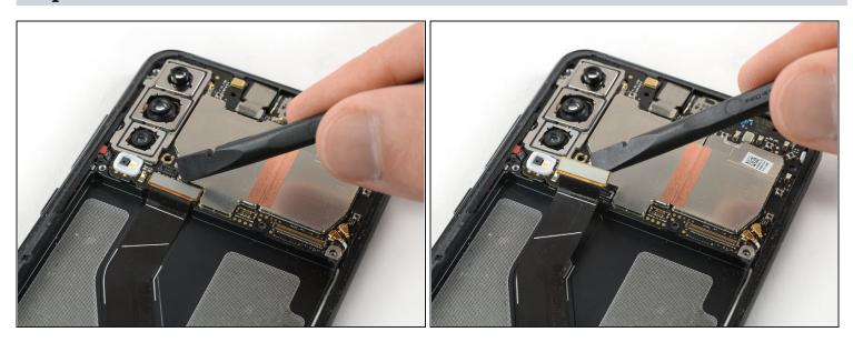
• Use the flat end of a spudger to pry up and disconnect the display flex cable at the bottom left of the motherboard.
