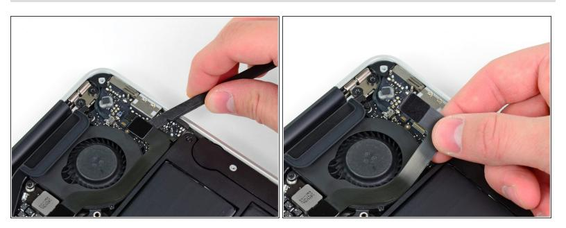
Use the flat end of a spudger to pry the I/O board cable connector upward out of its socket on the I/O board.
