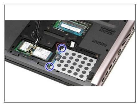
• Remove the screws that secure the hard-drive assembly to the computer.
