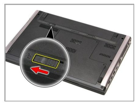
• Slide the other battery release latch to the unlock position.
