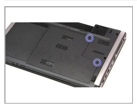
• Turn the laptop over and remove two screws securing the service cover.
