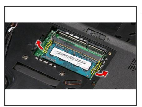
Push apart the memory retention clips to release the memory module.
