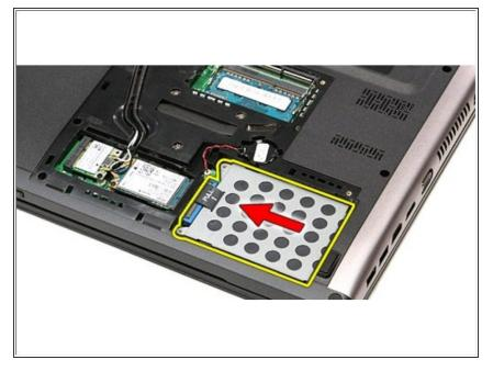
• Slide the hard-drive assembly towards the center of the computer.
