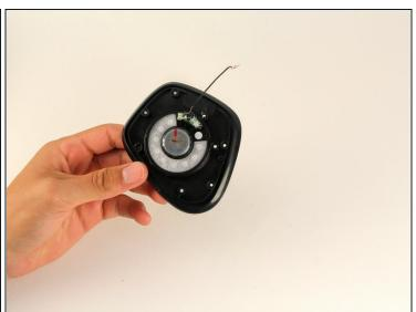
• Use a knife tool as a wedge to remove the speaker and glue in the new speaker.
