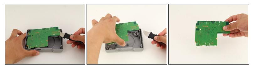
• Carefully remove the motherboard from the the rest of the console using your hands or the Jimmy tool.
