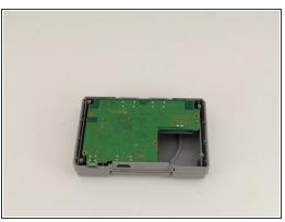
Remove the back plate from the rest of the console using your hands or the Jimmy tool.
