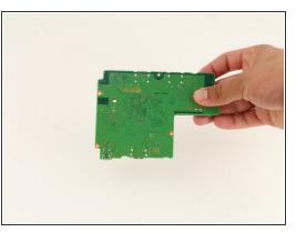
Carefully remove the motherboard from the the rest of the console using your hands or the Jimmy tool.
