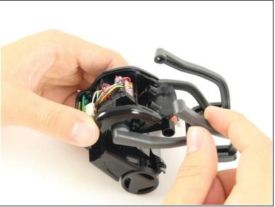
Gripping the shaft with needle nosed pliers, pull the opposite top arm off the main shaft.
