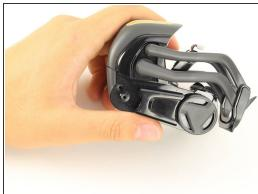
• Unscrew the two 2 mm body screws using a Phillips #0 screwdriver.
