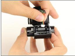
Gently unplug and remove the infrared sensor.
