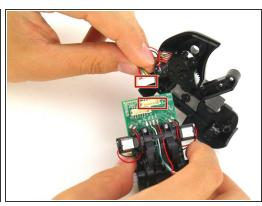
• Unplug the two motor connectors from the motherboard.
