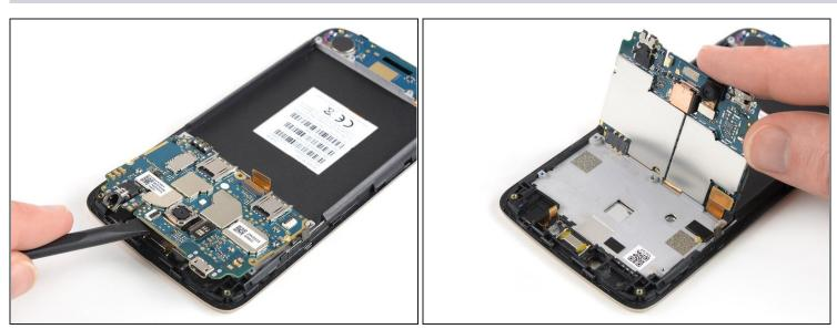
⚠ Don't try to remove the motherboard all the way yet. The display flex cable is still connected to its rear side.
