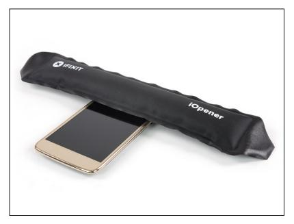
Use an iOpener and apply it to the top edge of the display to loosen the adhesive beneath the earpiece speaker.
