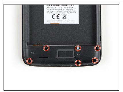
Remove the six 3.1 mm Phillips #00 screws securing the daughterboard cover.
