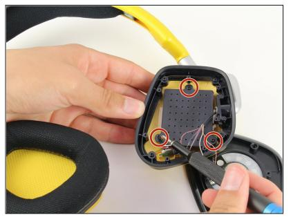
Using the Phillips #0 screwdriver, remove the three 6.4 mm screws on the black plastic panel with the grid of holes.
