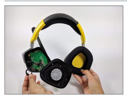
Pull the volume switch out and remove it from the device.
