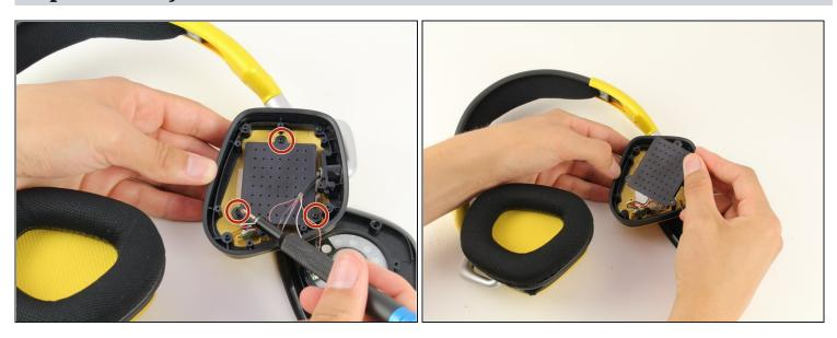
• Using the Phillips #0 screwdriver, remove the three 6.4 mm screws on the black plastic panel with the grid of holes.
