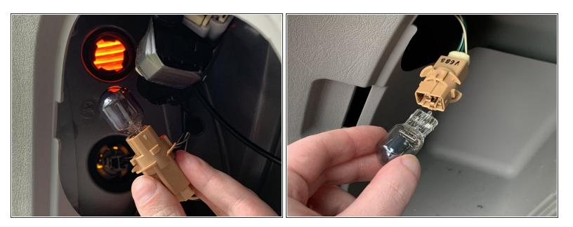
Hold onto the bulb socket and gently pull out the bulb with your other hand.
