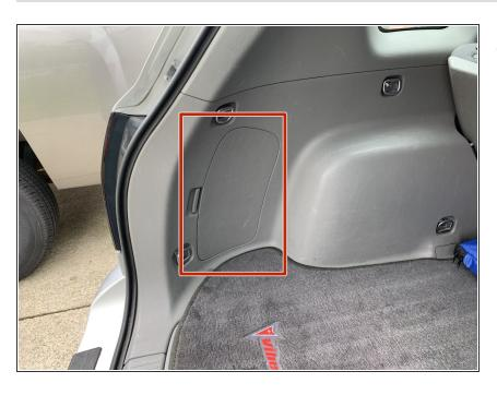
Locate the tail light access doors on the left and right sides in the trunk compartment.
