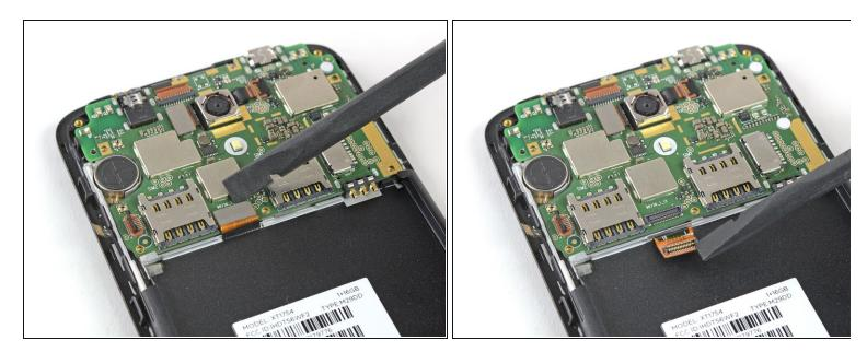
• Use the flat end of a spudger to pry up and disconnect the display flex cable located at the bottom of the motherboard.
