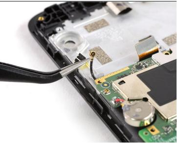
• Use a pair of tweezers to pry up and disconnect the antenna cable from the back of the motherboard.
