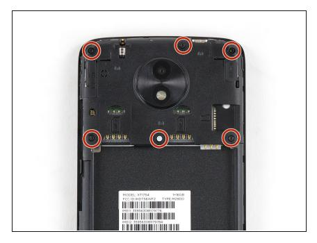
Remove the six 3.5 mm long Torx T5 screws.
