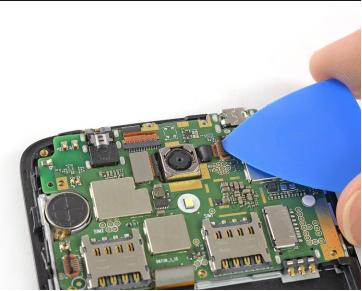
• Use the tip of an opening pick to pry up and open the black lever of the ZIF connector located at the top of the motherboard next to the rear camera.
