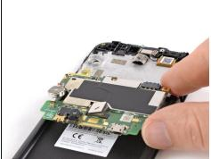
• Fold the motherboard over the battery cavity to access the coaxial cable connectors.
