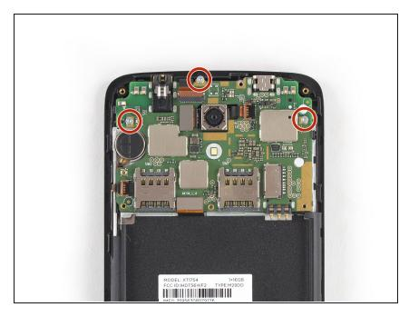
Remove the three 2.5 mm long T5 Torx screws.
