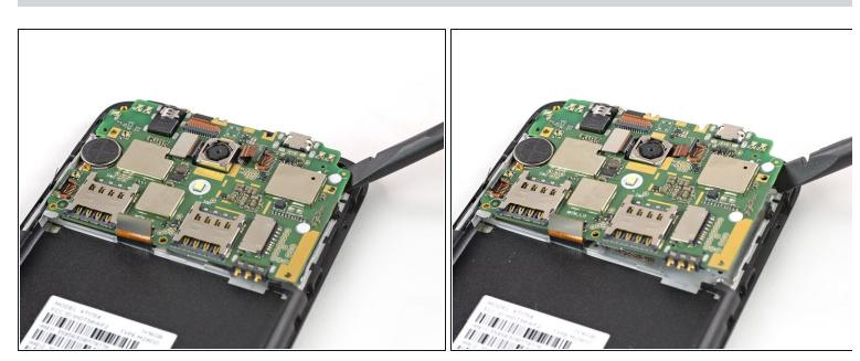
⚠ Don't try to remove the motherboard all the way yet. The antenna cable is still connected to its rear side.
