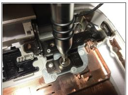
Dismount the display corners by removing the labeled 5.5 mm screws on the corners using a Philips #0 screwdriver to remove the screws.
