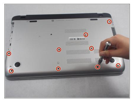
Using a magnetic screwdriver with a Philips #0 head, remove all of the visible screws on your laptop's bottom face. These screws are all about 7.5mm long.
