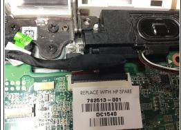
Notice that the motherboard is connected to multiple components of the computer that need to be disconnected first
