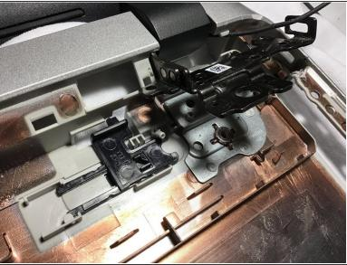
Notice after removing the screws the screen become able to move easily.
