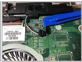
Use a plastic opening tool to separate the speaker's cable from the mother board, by pushing on the speaker's plugged cable
