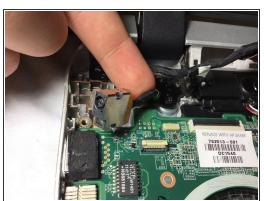
Remove the metal cover to free the motherboard supply cable.
