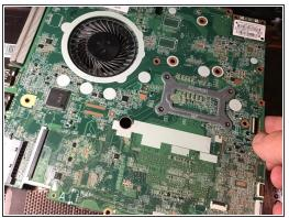
After the motherboard is dismounted and all the cable are disconnected, remove the motherboard from the device.
