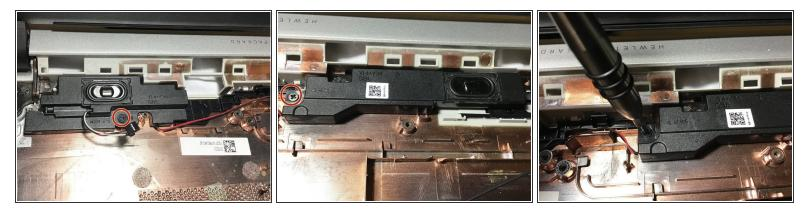
Dismount the speakers by removing the labeled 5.5 mm screws.
