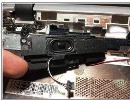
• Use a plastic opening tool to pry the left speaker out of it's place.
