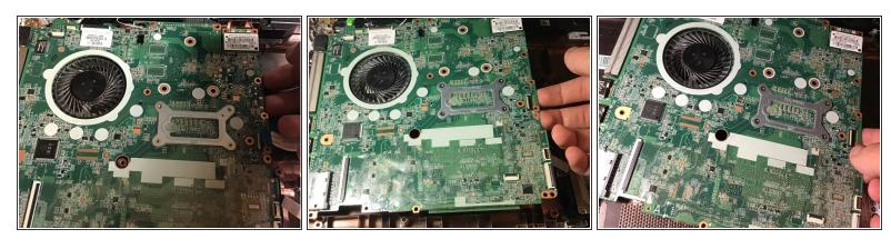
After the motherboard is dismounted and all the cable are disconnected, remove the motherboard from the device.
