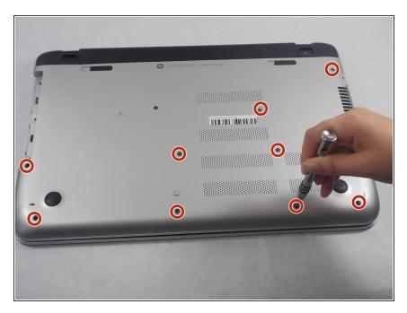
Using a magnetic screwdriver with a Philips #0 head, remove all of the visible screws on your laptop's bottom face. These screws are all about 7.5mm long.
