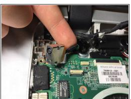
Remove the metal cover to free the motherboard supply cable.
