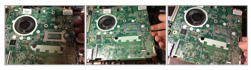
After the motherboard is dismounted and all the cable are disconnected, remove the motherboard from the device.
