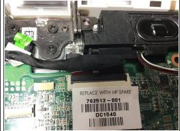
Notice that the motherboard is connected to multiple components of the computer that need to be disconnected first
