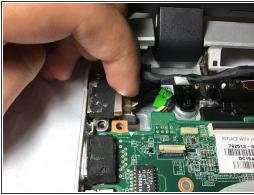
• Dismount the power supply cable holding the motherboard, by removing the 5.5 mm screws shown in the first picture on the right, using a Philips #0 screwdriver to remove the screws.
