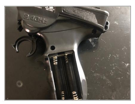
Unscrew all the screws using the Phillips screwdriver.
