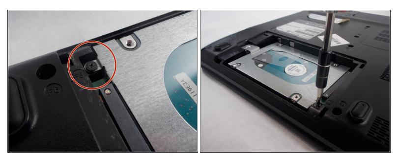
With a Phillips head screwdriver remove the final screw holding the hard drive in place.
