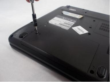
Using a Phillips head screwdriver, remove the one screw holding the backplate on.
