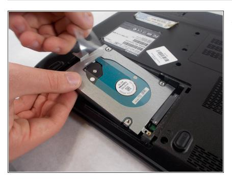
To remove the hard drive, lift up the plastic tap attached to it and slowly pull up using your other hand as support.
