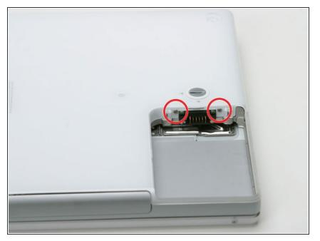
Remove the two 4.2 mm Phillips screws on either side of the battery contacts.
