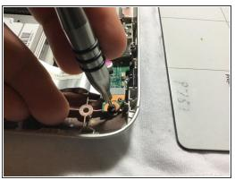
Using a magnetic screwdriver with a Philips #0 head, remove both screws that are holding down the circuit These screws are all about 5.5mm long.
