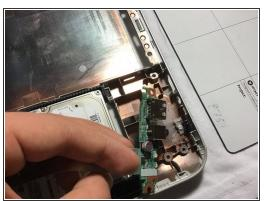
Once the circuit is unmounted gently remove the circuit board to be replaced.
