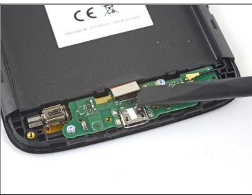
• Use a spudger to pry up and disconnect the motherboard flex cable connector from the daughterboard.
