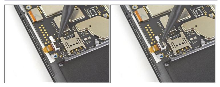
• Use the point of a spudger to lift up the locking mechanism securing the ribbon cable to the ZIF connector.
