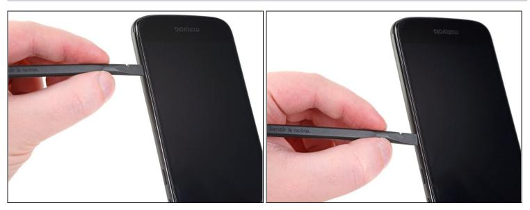
• Continue sliding your fingernail or spudger along the seam around the rest of the phone to release the remaining clips.
