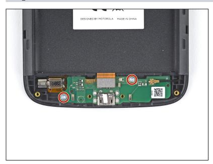
Remove the 3 mm-long T5 Torx screws securing the daughterboard to the phone's frame.
