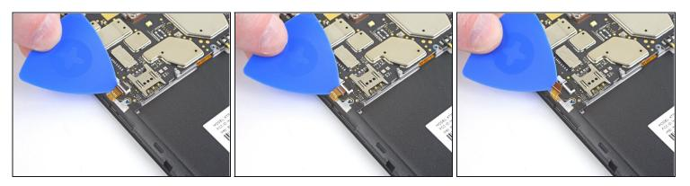
• Slide an opening pick between the ribbon cable and the motherboard to remove the cable from its connector.
