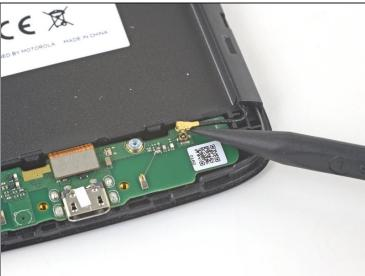
• Use the point of a spudger to pry up and disconnect the antenna cable from the daughterboard.
