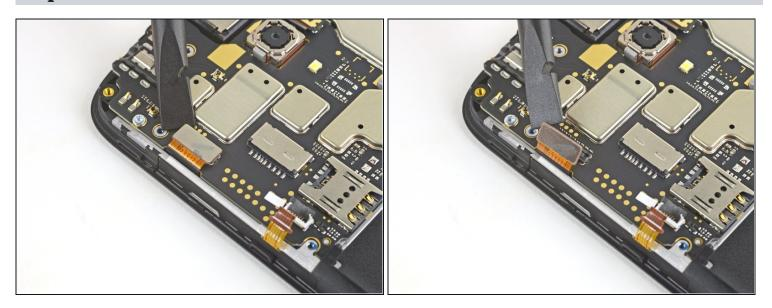
• Use a spudger to pry up and disconnect the display connector from the motherboard.
