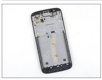
Only the frame and the LCD screen and digitizer assembly remain. Double-check that you removed all of the necessary components. Compare your new replacement part to the original part—you may need to transfer remaining components or remove adhesive backings from the new part before installing.
