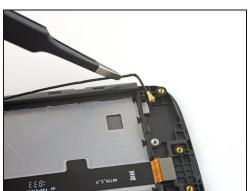
• Use your fingers or a pair of tweezers to lift and de-route the antenna cable from its groove on the right edge of the phone.
