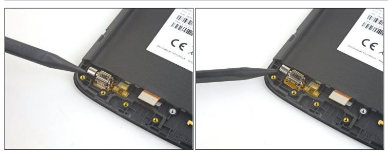
• Use the point of a spudger to pry up and loosen the vibration motor from its recess.
