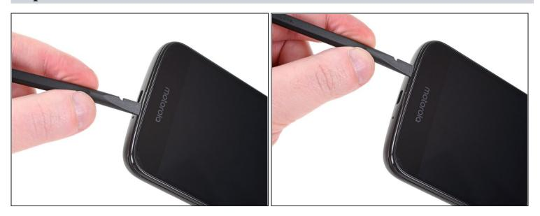
• Insert your fingernail or the flat end of a spudger into the seam on the bottom of the phone and slide it along the edge to release the clips holding the back cover to the phone.
