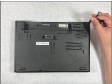
• Use a Phillips #1 screwdriver to remove the two 9mm screws holding the back cover.
